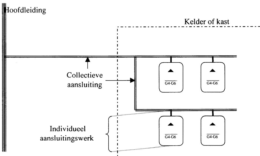
Schema nr. 2 – Aansluiting > 8 meter
